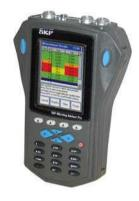
The SKF Microlog CMXA75 kit for railway comes as a complete kit that includes Microlog, software, vibration sensors and cables. In railway workshops the Microlog can be used to check drives and wheelset bearings during the wheel reprofile process. In train operation service it can be used to troubleshoot various bogie subsystems including traction motors, gear boxes and wheelset bearings. Benefits include:
