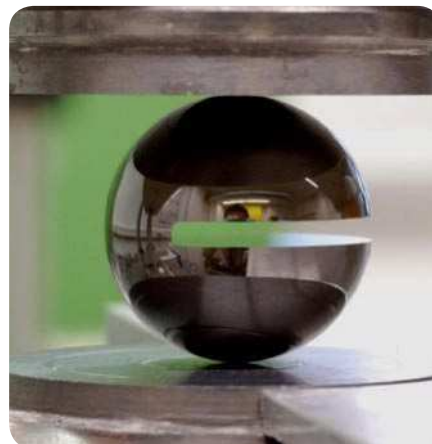
“Notched ball” test for ceramic balls
