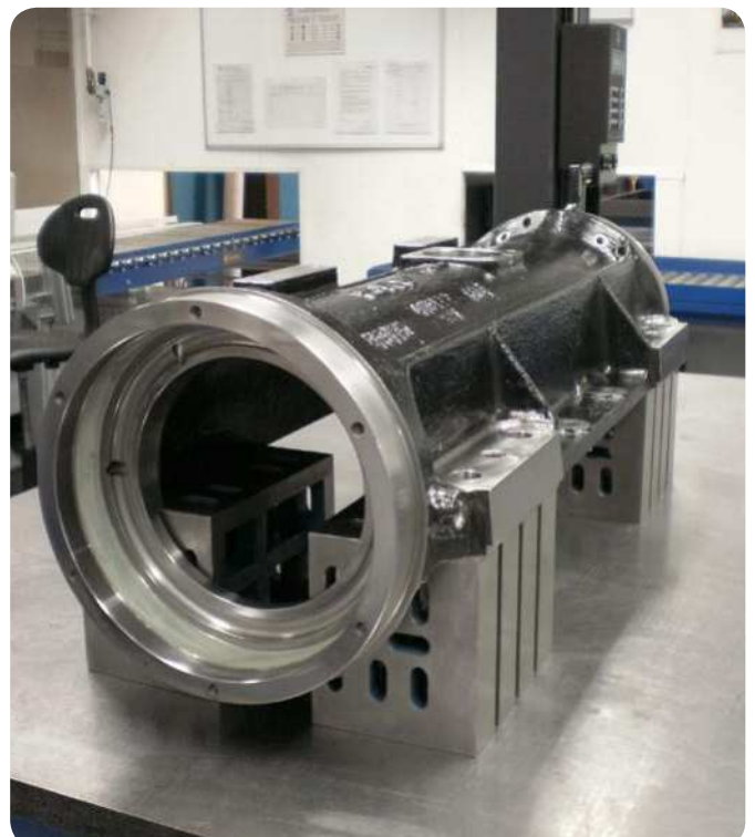
SKF suspension tube ready for shipment A glass fibre sleeve is fitted to the bore, which enables easy bearing replacement during remanufacturing, if needed.
