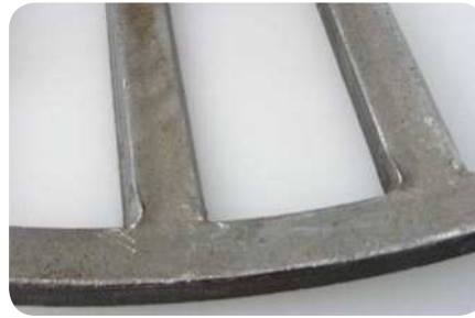
Abrasive wear Abrasive wear on a steel cage of a tapered roller bearing
