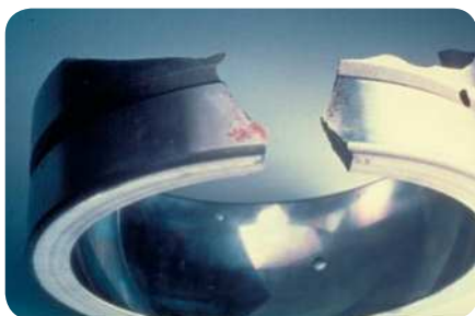
Forced fracture Bad housing seat, finally resulting in a cracked outer ring
