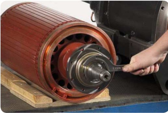
Step 7: Securing the TMBU in the axial direction with a lock nut
