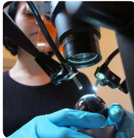
Optical testing of the ball surface
