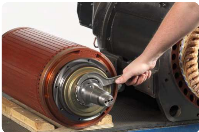
Step 4: Securing the TMBU in the axial direction with a lock nut
