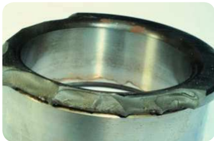
Forced fracture Cracked flanges of a cylindrical roller bearing inner ring due to impact load
