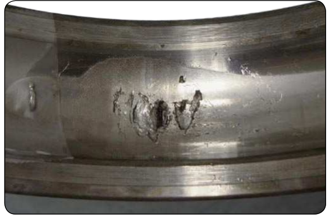
Excessive voltage Ball bearing raceway with large spalls
