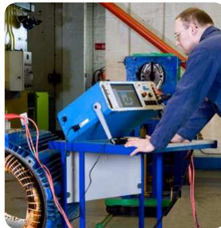
Static testing of an AC stator
