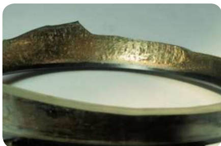
Fatigue fracture Fatigue fracture of a spherical roller bearing outer ring
