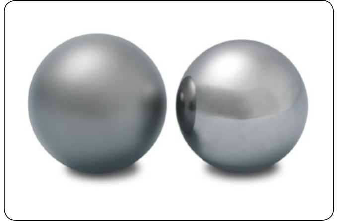
A dull grey surface of the rolling elements can be a sign of microcratering.
