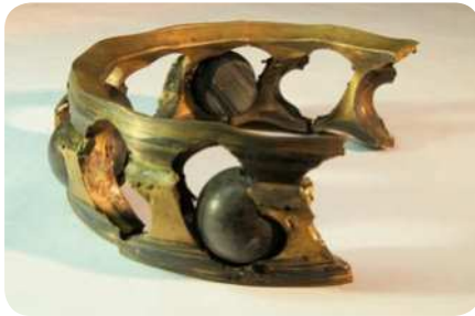
Failure of a cage and roller assembly of a deep groove ball bearing of a traction motor.
