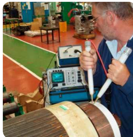
Static testing of a DC rotor
