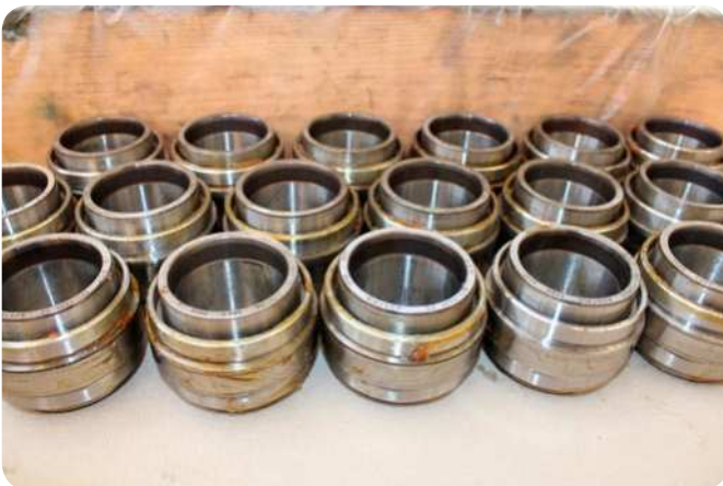
Remanufacturing of traction motor bearing units Disassembled bearings, inner ring assemblies ready for inspection of the condition of the grease prior to cleaning
