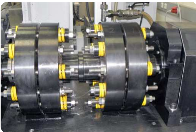
Endurance life test rig with two sets of four axially loaded hybrid angular contact ball bearings
