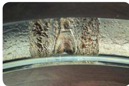
Subsurface initiated fatigue
