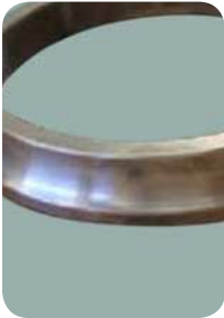
Four-point contact ball bearing inner ring with damage
