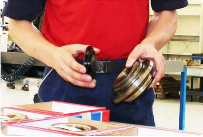
Remanufacturing of traction motor bearing units Discarding the transportation protection
