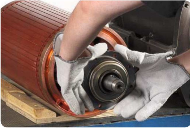
Step 6: Installing the non-locating bearing unit
