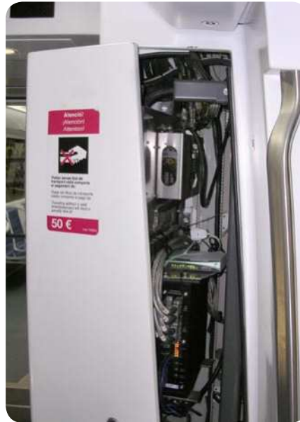
Metro Barcelona coaches in different trains are equipped with condition monitoring units
