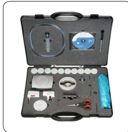
SKF portable grease analysis kit for field use
