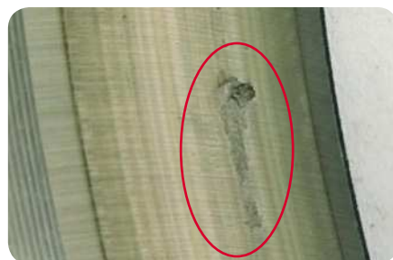
Surface initiated fatigue
