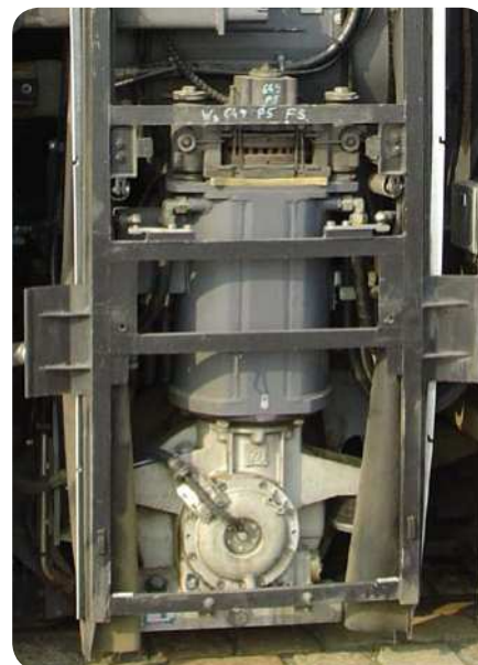
Vertical drive system for single-wheel system used for low-floor light rail vehicles
