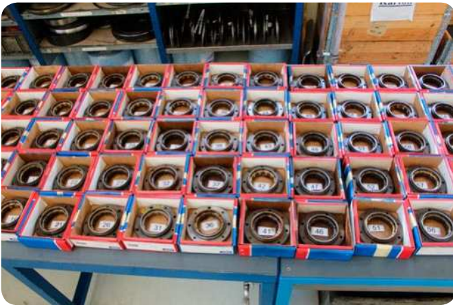
Remanufacturing of traction motor bearing units Disassembled bearings, outer rings with cage and roller assembly, ready for inspection of the condition of the grease prior to cleaning
