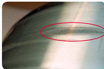
Adhesive wear Adhesive wear on the inner ring raceway of a cylindrical roller bearing
