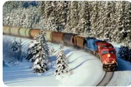
American diesel-electric locomotives are typically hauling very long freight trains, total power rating 2 200 kW (3 000 HP) up to 4 500 kW (6 000 HP).
