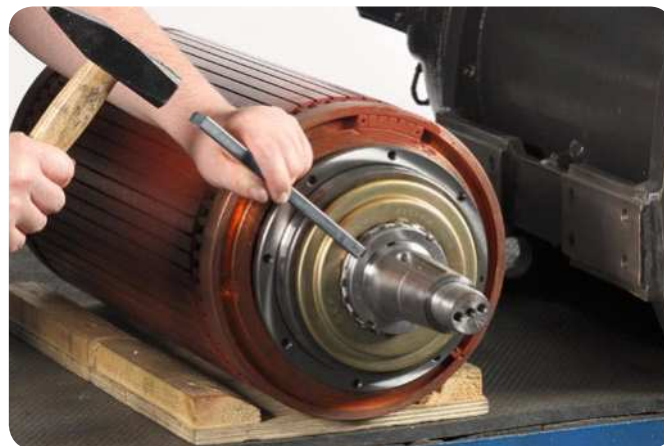
Step 5: Securing the locknut by bending one of the locking washer tabs
