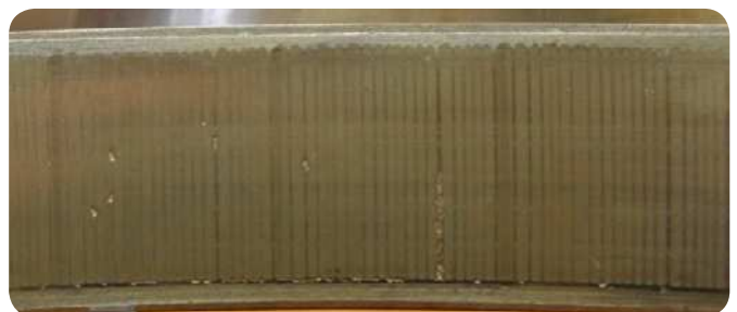
Fluting or washboarding in a raceway caused by the passage of damaging electrical current.
