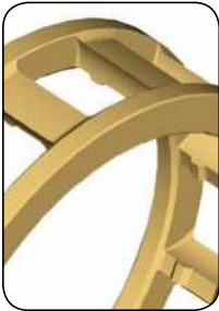
One-piece machined brass cage, outer ring centred, designation suffix ML
