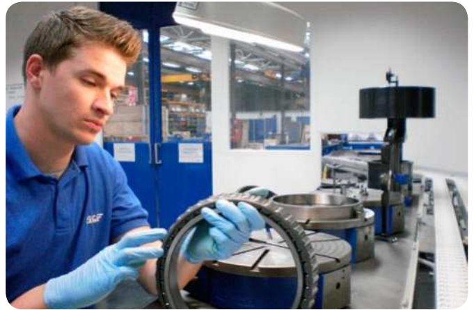
Remanufacturing of tapered roller bearings for suspension tubes Inspection of the condition of the cage and roller assembly after cleaning
