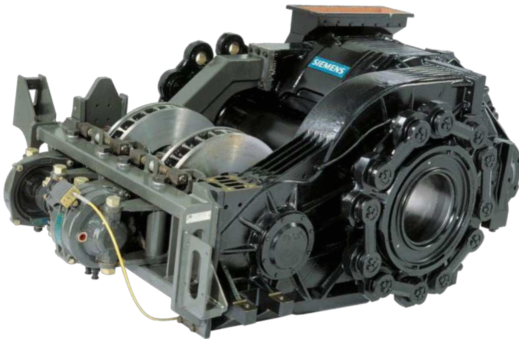
High-speed quill drive design with integrated disc brake shaft Source: Siemens
