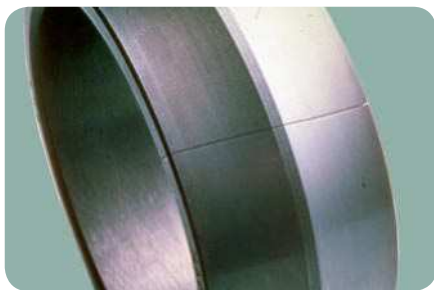
Forced fracture Forced fracture through excessive drive-up
