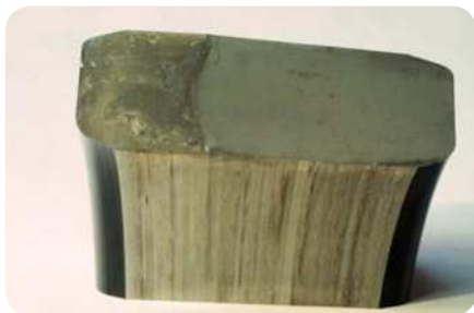
Forced fracture Cracked inner ring of a cylindrical roller bearing
