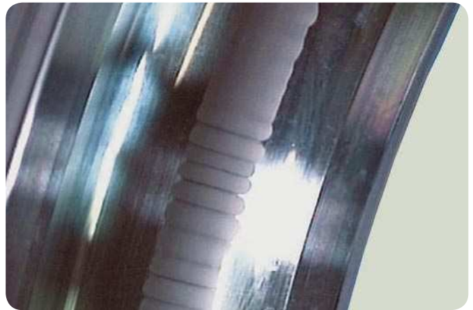
Fluting or washboarding in a raceway caused by the passage of damaging electrical current.
