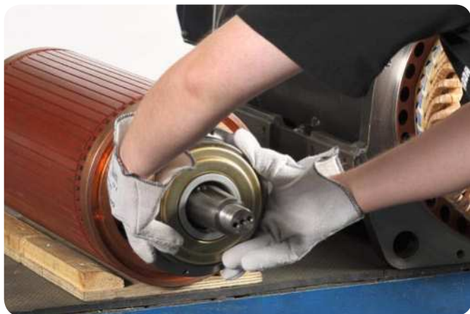
Step 3: Installing the locating TMBU
