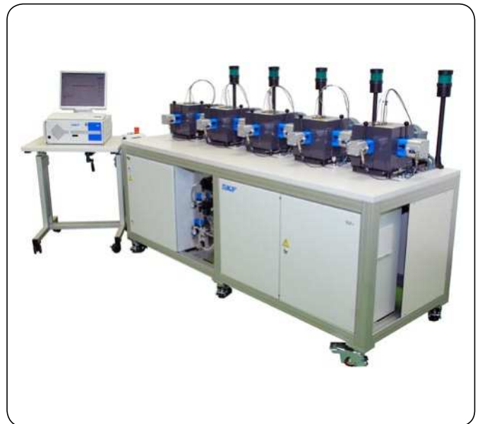
SKF grease test rig used to determine the most suitable grease quality
