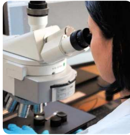
Checking macrostructure, microstructure and homogeneity on sectioned samples
