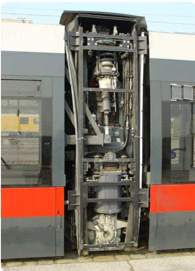
Vertical drive system for single-wheel system used for low-floor light rail vehicles
