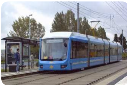
German Chemnitz Variobahn light rail vehicles max. speed 70 km/h, hub traction motor drive system (→ chapter 2), power 8 x 45 kW 3) , in operation since 1998, prototype since 1993 [4] .
