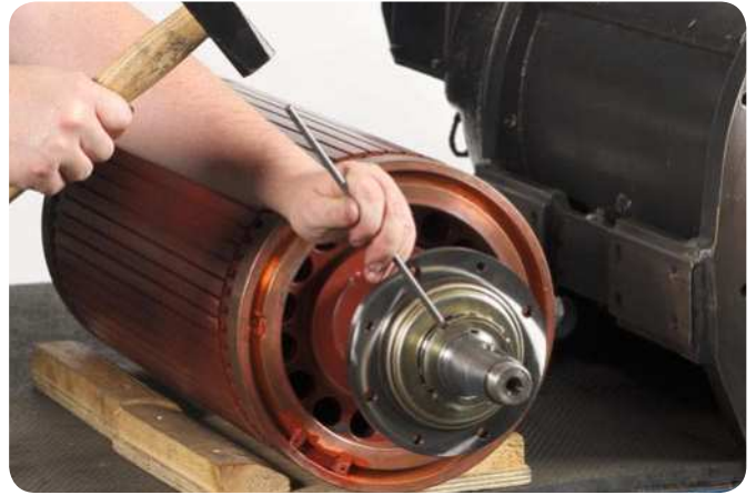
Step 8: Securing the locknut by bending one of the locking washer tabs
